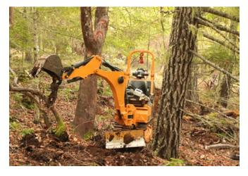
commercially viable way. The machine's 6-way dozer blade, 32-horsepower engine, and 24-inch minimum width get tough jobs done in tight spaces—and with full remote controls so the operator can be in the seat or up to 150 feet away.
